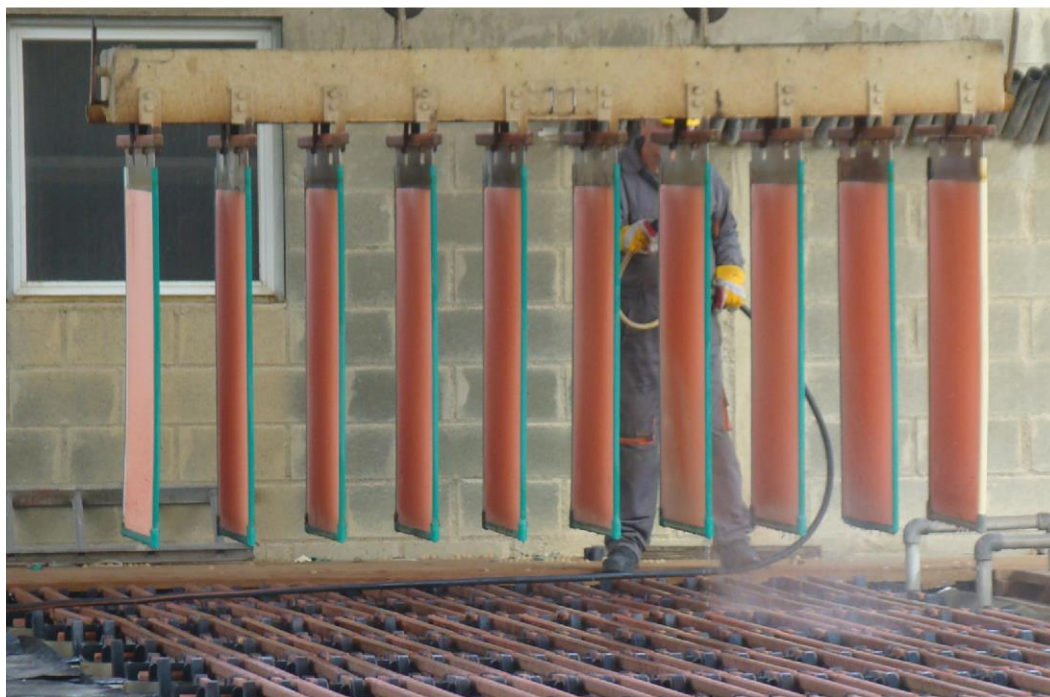
Figure 3: Pure copper plates exiting the electrolytic vat in a cypriot mine. The state of surface is highly rough and scatters the ambient light so the leftmost plate appears light pink. The other plates facing each other appear orange in such lighting conditions (the direct solar light is screened by the shed roof) and a greyish diffuse environment.
